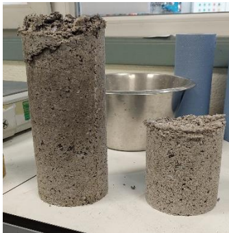
RECQB2 - Vibrocompaction test
